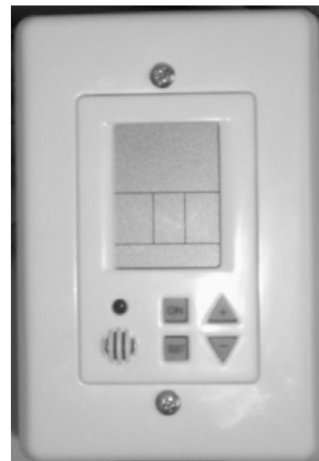
Figure 5 – Remote Thermostat Control
