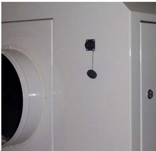
Figure 4 – Remote Thermostat Connection
